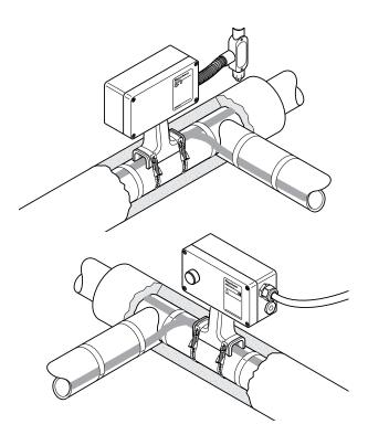
The JBM-100 kit is designed to connect power to up to three Raychem BTV, QTVR, XTV, KTV, or VPL industrial parallel heating cables and is approved by FM, CSA, and PTB for use in hazardous locations.
